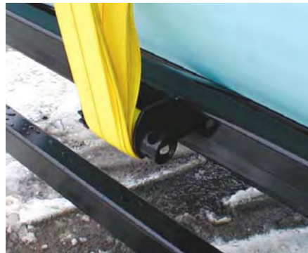
Nylon Tie Down straps secures tank to the trailer. Winch mounts are permanently welded to the trailer as well.
